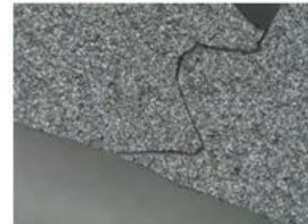
Physical Match of Paint Chip Edges
